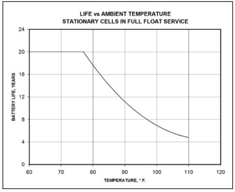
FIGURE 4.1.4 - Battery Life versus ambient temperature
