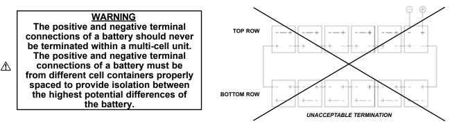
If there are an even number of tiers or steps, the battery will terminate on a common end. If there are an odd number of tiers or steps, the battery will terminate at opposite ends. Polarities below are shown for reference only.
