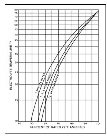
FIGURE 4.1.3 - Battery capacity versus operating temperature.
