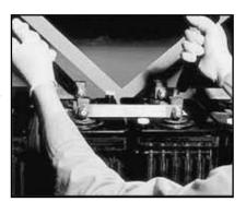
FIGURE 4.1.7 Measuring connection resistance with DLRO
