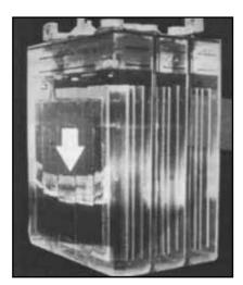
FIGURE 4.2.4 - Arrow points to white, crystalline hydrate
