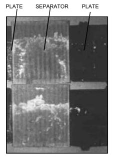
FIGURE 4.2.5 - Cutaway shows clogged separator with the by-products of hydration
