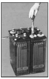
FIGURE 2.6.1 - Taking a hydrometer reading
