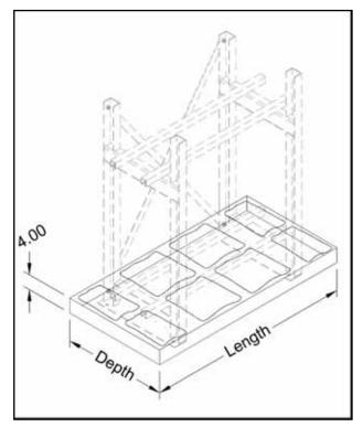
FIGURE C.1 - Spill containment barriers with pillows
